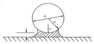
Figure 3 capillary force diagram
