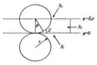
Figure 4 dust particles contact model
