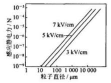
Figure 5 The relationship of induction electrostatic force, the particle diameter and ppliedvoltage
